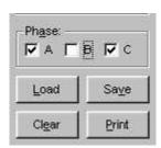
When the transient list is executed, the status of these phase check marks is incorporated in the generation of the list data sent to the AC Source unit.
